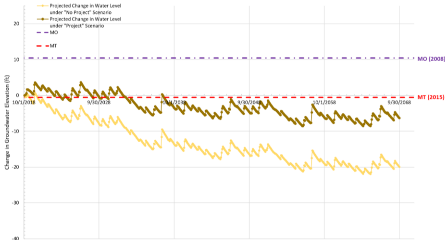
Figure 9-16. Comparison of Groundwater Elevation Changes Under Marina-Ord Water Augmentation “Project” Scenario and “No Project” Scenario, with MO Boundary Condition and 2030 Climate Condition
